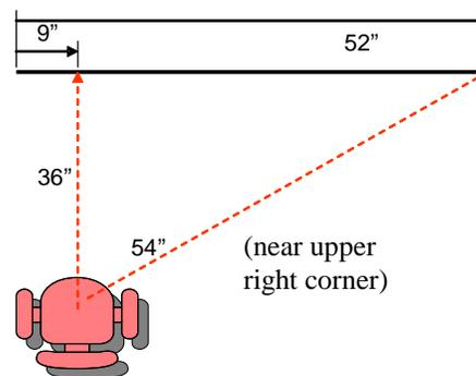
**Figure 4: Layout of Simulator Screen and Subject Positioning**
