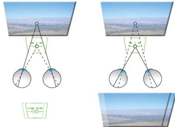
**Figure 1. Graphical Depiction Of Diplopia Caused By Concentrating On Two Objects At Different Distances Simultaneously. Concentrating On The OTW Scene (Shown To The Left) Causes A Diplopic Image Of The Reticle. Concentrating On The Reticle Image Of The Reticle Causes A Diplopic Image Of The OTW Scene.**
